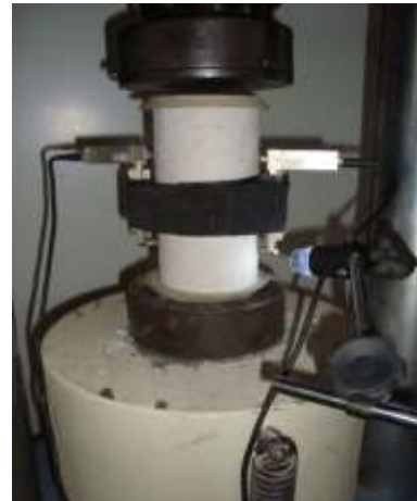
Figure 4 - Real setup of the experiment using a servo-hydraulic machine EMIC, Model PC 200 and an USB microscope (800x). The sample is also affixed with traditional strain gauges (mechanical extensometer).
